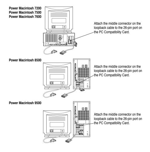
**WARNING** Do not plug a monitor into the joystick port marked with the icon  $\triangleq$  that comes on some models of the PC Compatibility Card, and do not plug a joystick into a monitor port (marked with the icon  $|\Box|$ ). Serious damage can result to your equipment.
