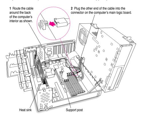
If there is a processor card in your computer, route the cable between the processor card and the back panel (not over the top of the processor card).
