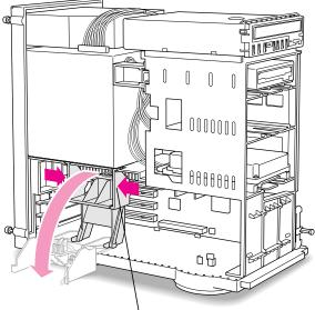
To lower the retainer, squeeze the sides to unlatch it.
