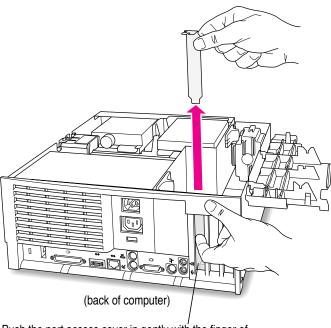
Push the port access cover in gently with the finger of one hand while pulling it straight up with the other hand.
