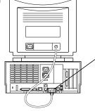
Attach the monitor cable to the built-in monitor port on the back of your computer.
