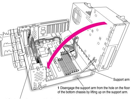
**2** Gently swing the top part of the chassis down until it rests securely on the bottom chassis. Be sure that you don't pinch any of the cables between the top and bottom parts of the chassis.
