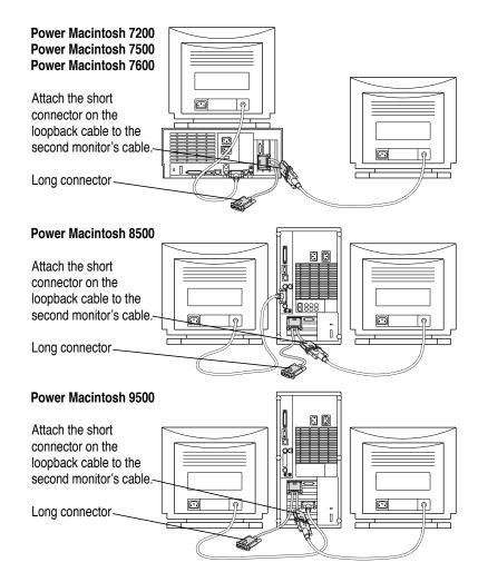
In most cases, you leave the long connector on the loopback cable unplugged. But if your computer has an additional video card or monitor port, you can plug the long connector into it. This will allow you to switch the monitor between the PC environment and the Mac OS environment.
