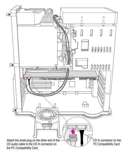
15 Plug the other end of the second cable into the CD In connector on your PC Compatibility Card.
