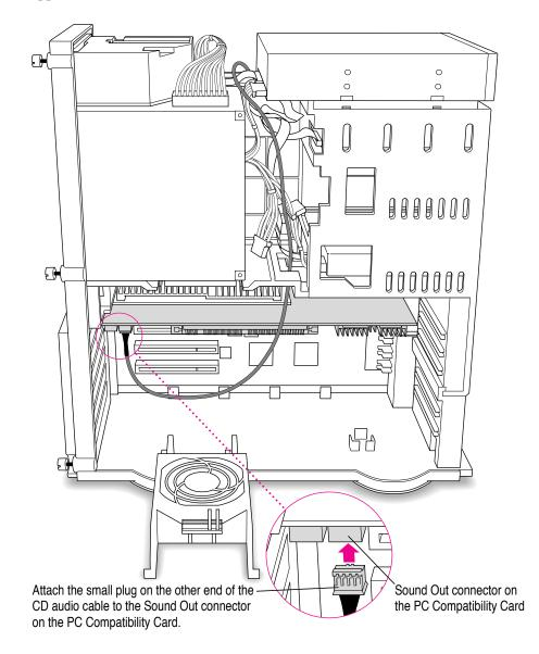
Installing the Card in a Power Macintosh 8500 or 9500
