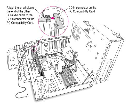
21 Route the second cable over the top of the card, around the back of the logic board, and through the hole in the computer's chassis.
