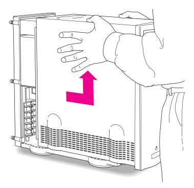
4 Touch the metal part of the power supply case inside the computer to discharge static electricity.
