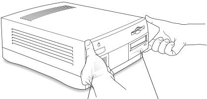
Locate the two release buttons under the front panel ledge with your fingertips.
