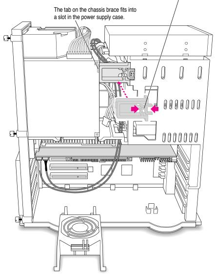
Squeeze here, and reinstall the chassis brace. Be sure not to pinch any of the cables between the chassis brace and the power supply case.
